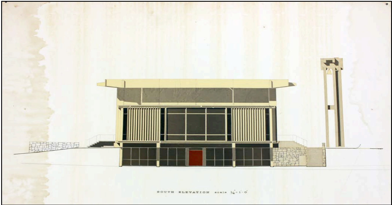
Image 11: South Elevation, Presentation Board, ca. May 1960, Charles M. Goodman Associates. This presentation board focuses on the south elevation of the unbuilt Social Hall, with the roofline and clerestory windows of the main Sanctuary visible behind. The Social Hall was designed as complementary, but not identical to the main block, with a lower-set roofline, broader expanses of fixed glass at the first story level, and wrapping fixed windows at the ground level. The unbuilt bell tower is also visible in the background. From the Archives of the Unitarian Universalist Church of Arlington.
