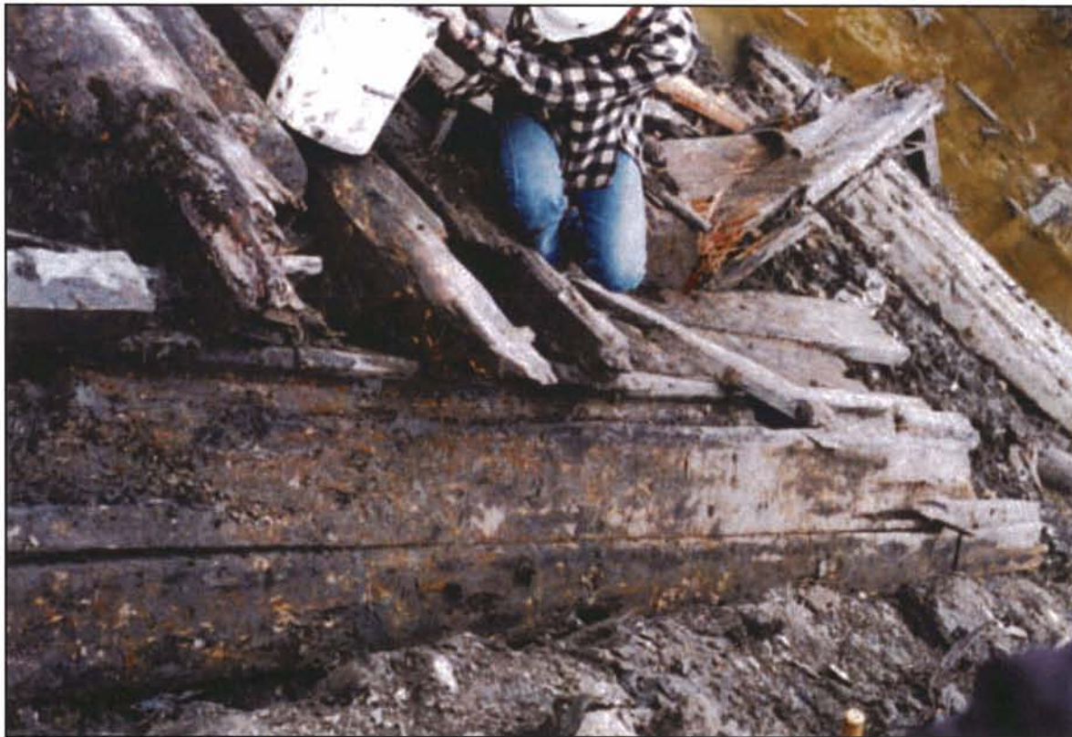
Figure 32. Forward section of the keel and false keel with sheathing.
