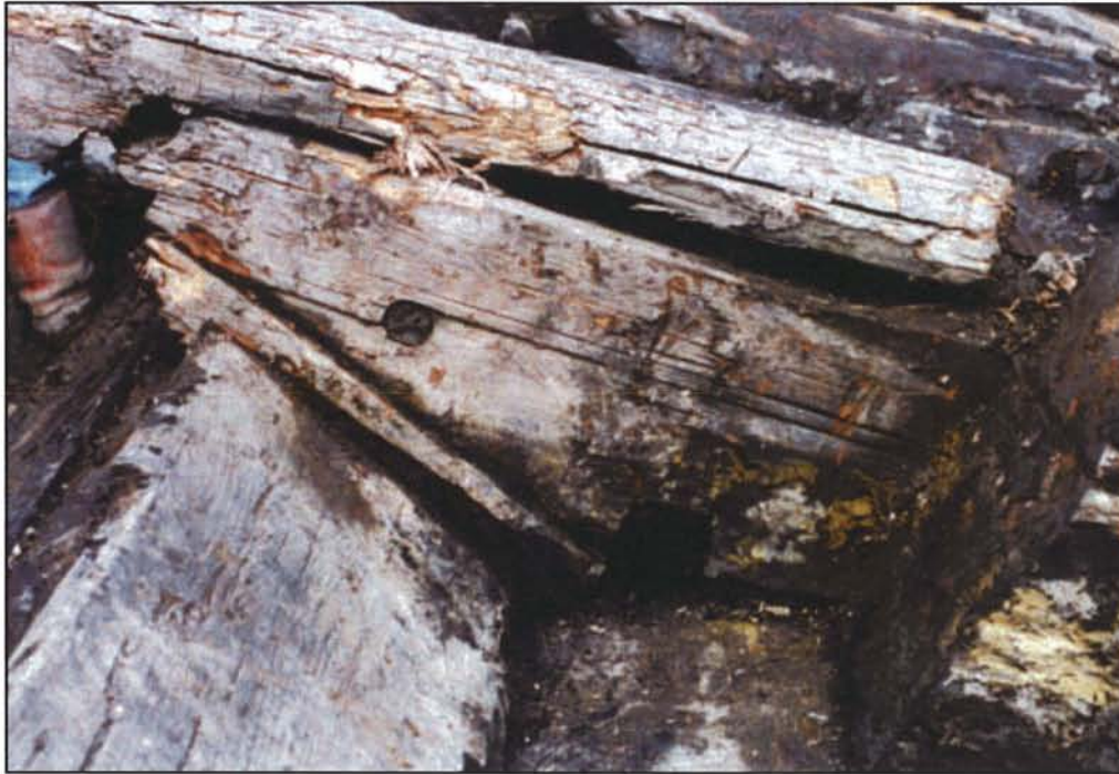
Figure 29. Forward section of the keel showing rebates for the floors and the starboard garboard strake.
