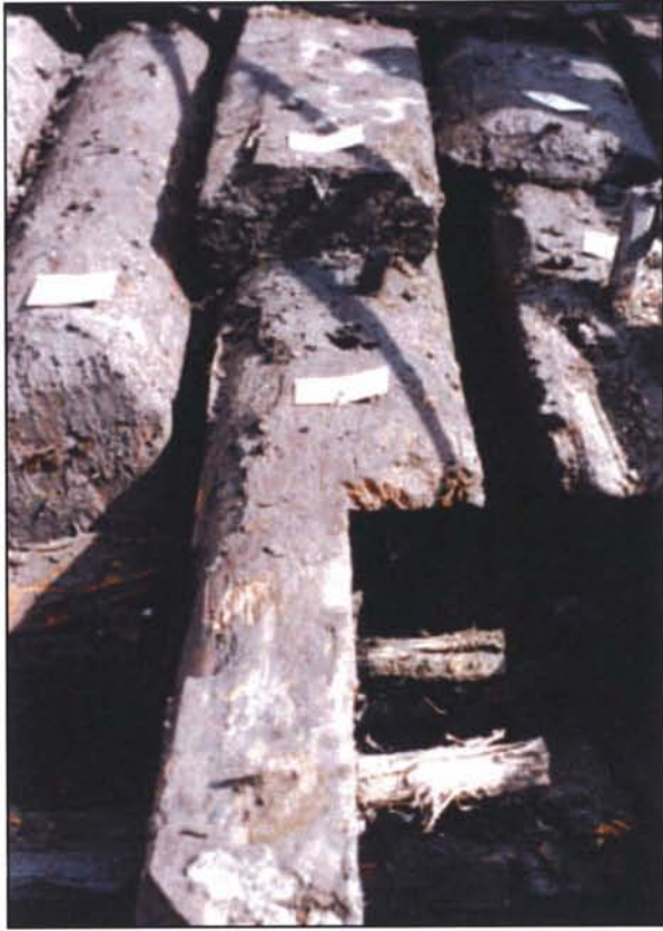
Figure 40. Scarf in a starboard half floor to accept a port half floor.
