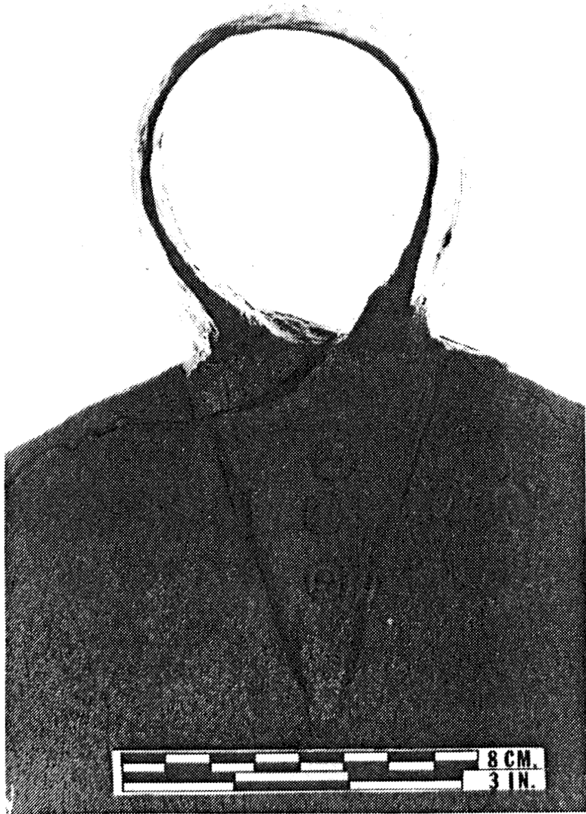
Figure 17. Lap weld seam in Type II hoe. Front view of hoe collar and spine.
