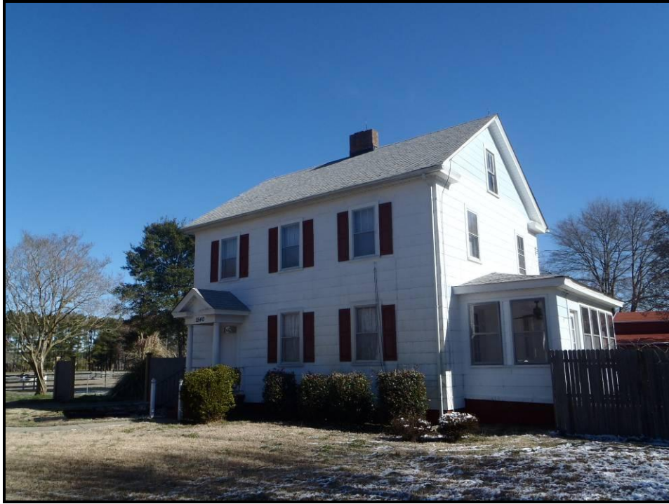
Figure 29. Example of Two-Story Side Hall Plan Dwelling (VDHR #131-0106), 1540 Benefit Road, View Looking Northeast.
