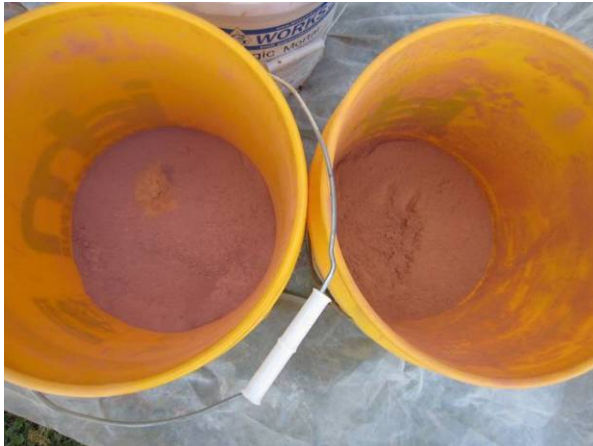
(Left) Two shades of brick patching mortar were used. (Right) Patching the glazed header with Jahn repair mortar.
