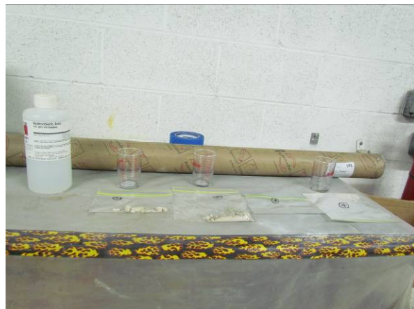
(Left and right) Performing a basic mortar analysis in house by means of acid digestion.
