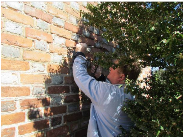
(Left and right) Removing samples of mortar from the wall and arch of the south elevation.
