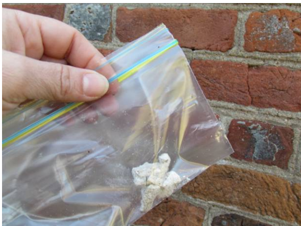
(Left and right) Performing a basic mortar analysis in house by means of acid digestion.
