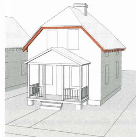
Exposed rafter ends
