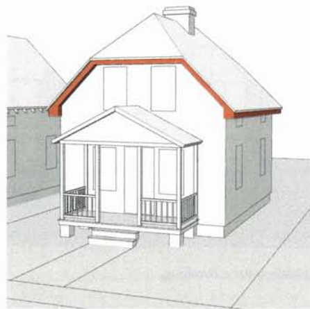
Boxed-in rafter ends
