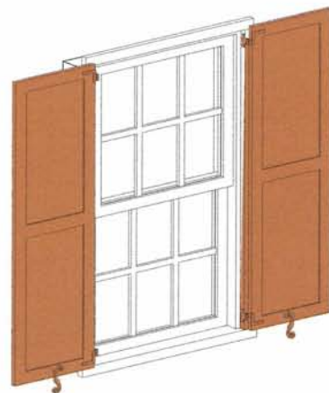
Properly mounted shutters have upper and lower hinges and are kept open with shutter dogs.
