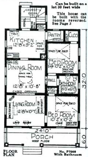
FLOOR PLAN No. P7009 With Bathroom
