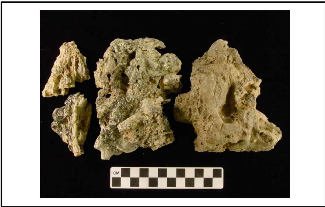
THE OTTERY GROUP 2900 Linden Lane, Suite 21C Silver Spring, MD 20910 phone (301) 562-1975 fax (301) 562-1976 www.otterygroup.com FIGURE 7.3 Example of Kiln Brick (Top) and Glaze Slag (Bottom)
