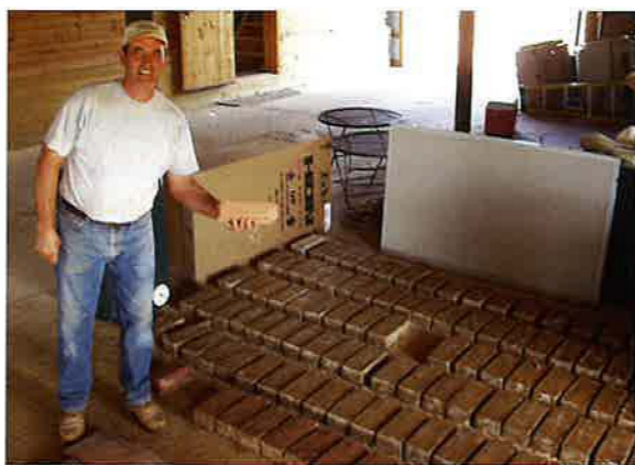
Bill Payne shows off a batch of some 60 bricks he molded from clay excavated on the plantation’s grounds. Payne set the bricks out to air-dry under shelter for about 30 days before firing them in an electric kiln for 8 hours at temperatures reaching 2,000 degrees Fahrenheit. The brownish-yellow clay used to make the bricks burns to a bright reddish orange when fired. Firing also shrinks the bricks considerably, but does so uniformly in an electric kiln. (Photo: Courtesy of Shirley Plantation)
