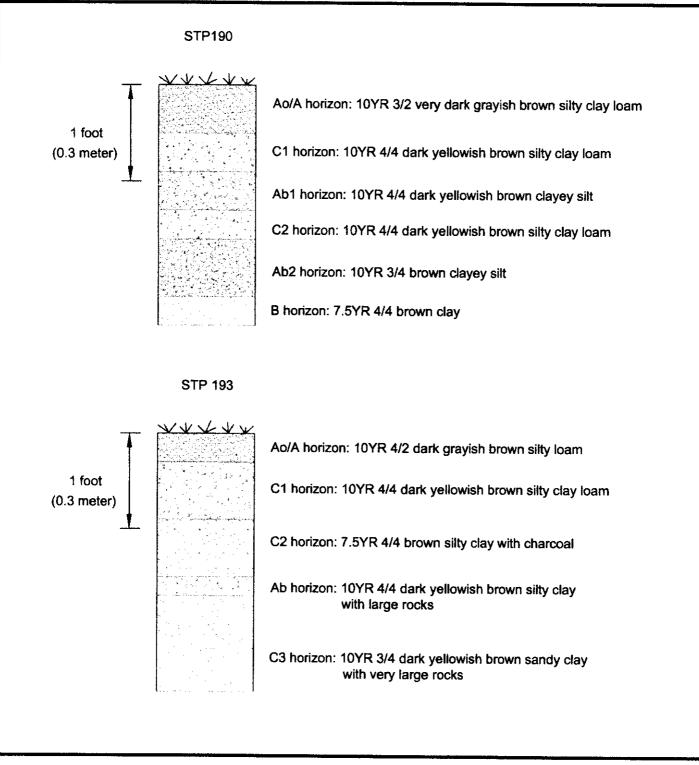
Soil Profiles from STP 190 and STP 193 44LD238/Structure 53-365 (Francis/Gulick Mill) Scale 1" = 1'
