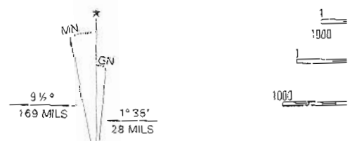
UTM GRID AND 1999 MAGNETIC NORTH
