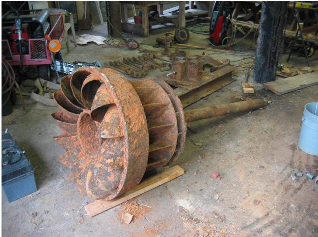
Mill Turbine During 2010 Refurbishing Project
