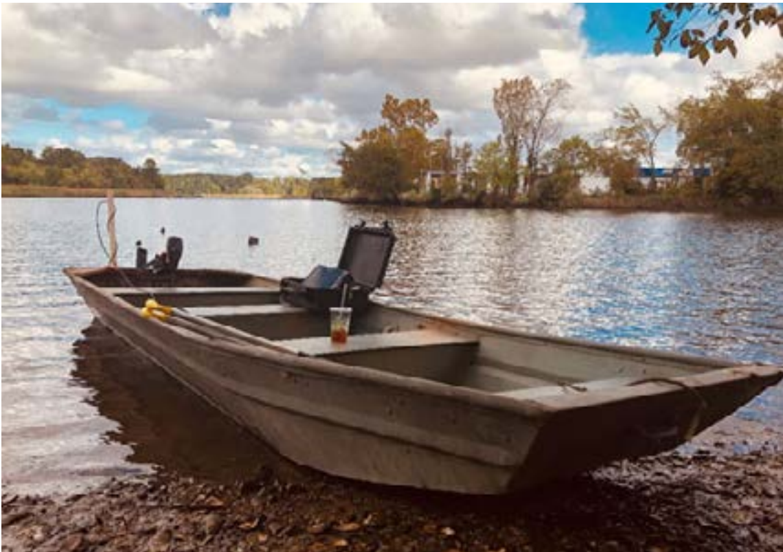
Figure 4. The R/V Nansemond rigged for side- imaging sonar. It used a 30-lb thrust trolling motor for propulsion and a secondary 12VDC battery to power the sonar unit. Positioning was acquired using a built-in GPS antenna and only collected with an HDOP of <1.1.
