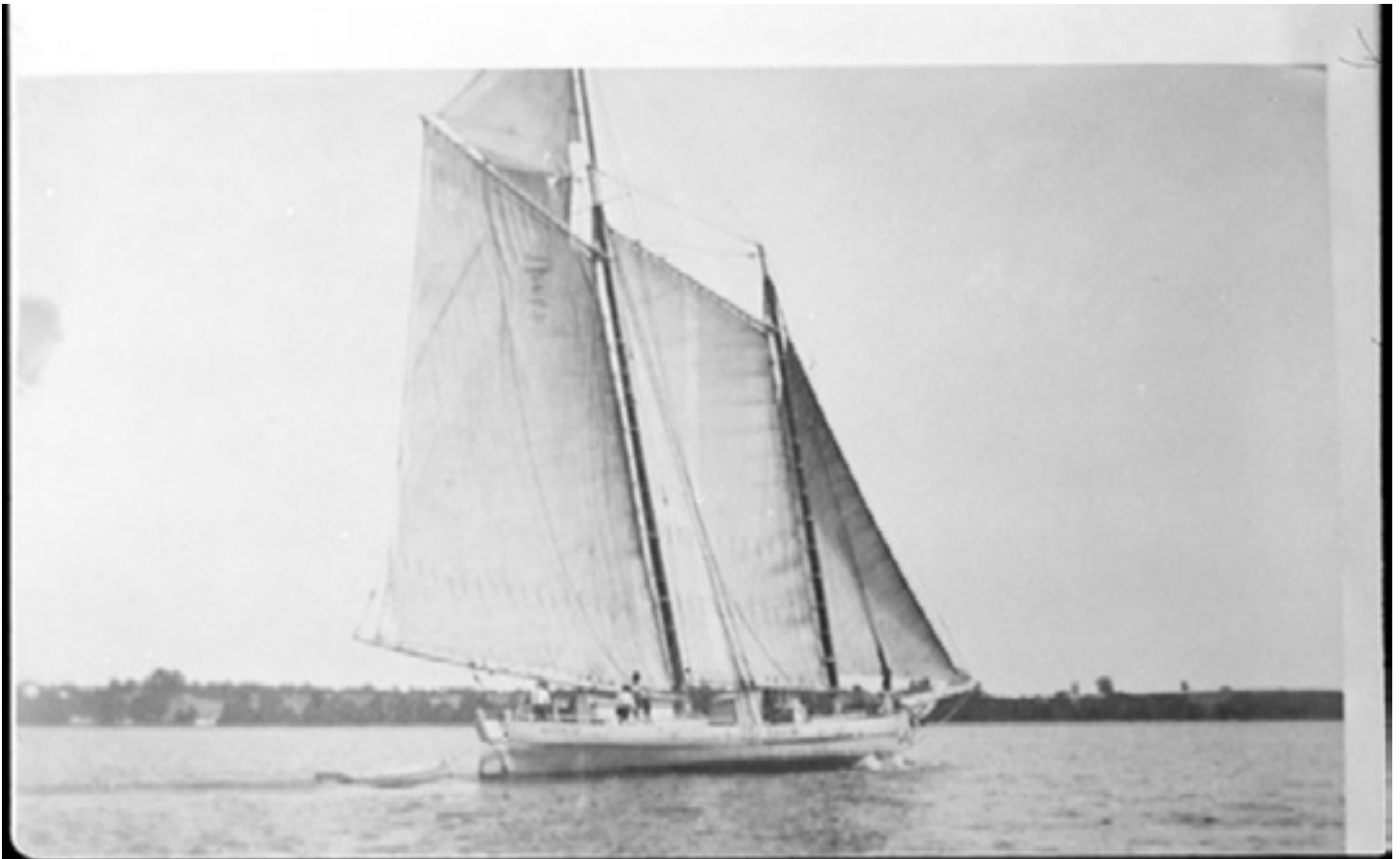
Figure 46. Inset of photograph taken by George Barrie in 1904 showing a square-rigged bugeye. Note the gaff-rigged sails and double-ended hull. This was one of only 37 known square-rigged bugeyes to be constructed. (Courtesy, Mariners' Museum)
