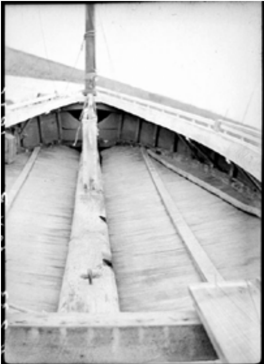
Figure 42. Inset of photo taken by M. V. Brewington of a crabbing skiff interior during a 1937 survey of Chesapeake Bay craft. Note the cross- planked interior, similar to planking recorded in Feature 10.
