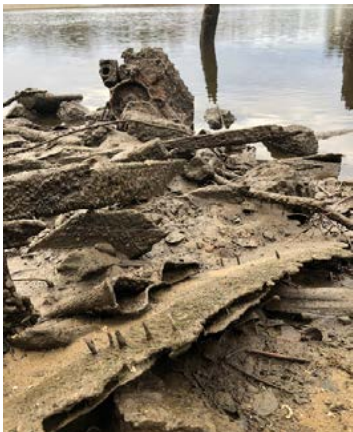
Figure 55. Detail of the Feature 13 boat. Note two layers of diagonally-laid planks and copper-alloy screws at frame stations. A frame is seen in the middle left-hand side of the picture and the engine is in the background.
