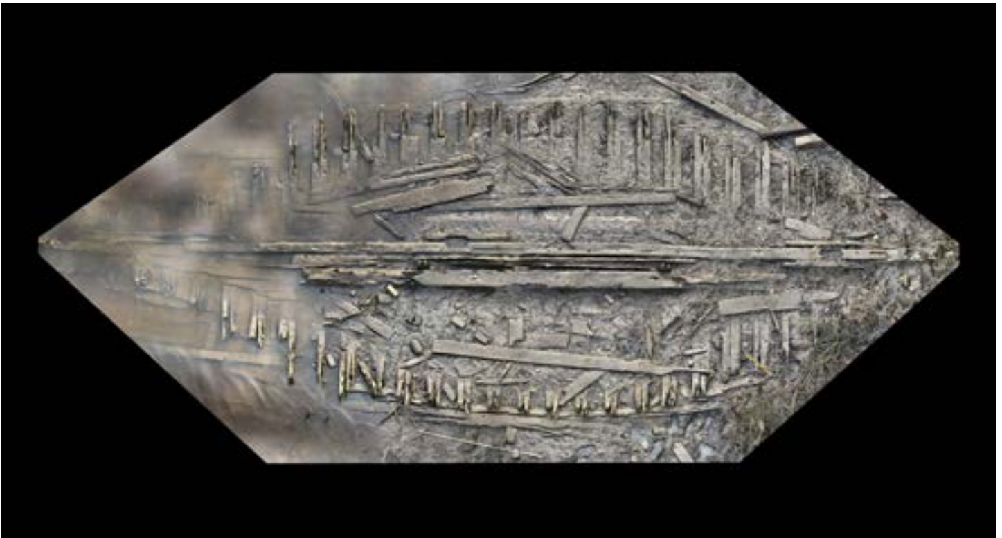
Figure 47. The Hobbs Wreck, Feature 11, shown in orthoimagery. The bow is oriented to the right in this photo and north is to the left. Note the mainmast step, located ahead of the aftermost extent of the centerboard trunk. This feature indicates a schooner, or square-rigged, bugeye.
