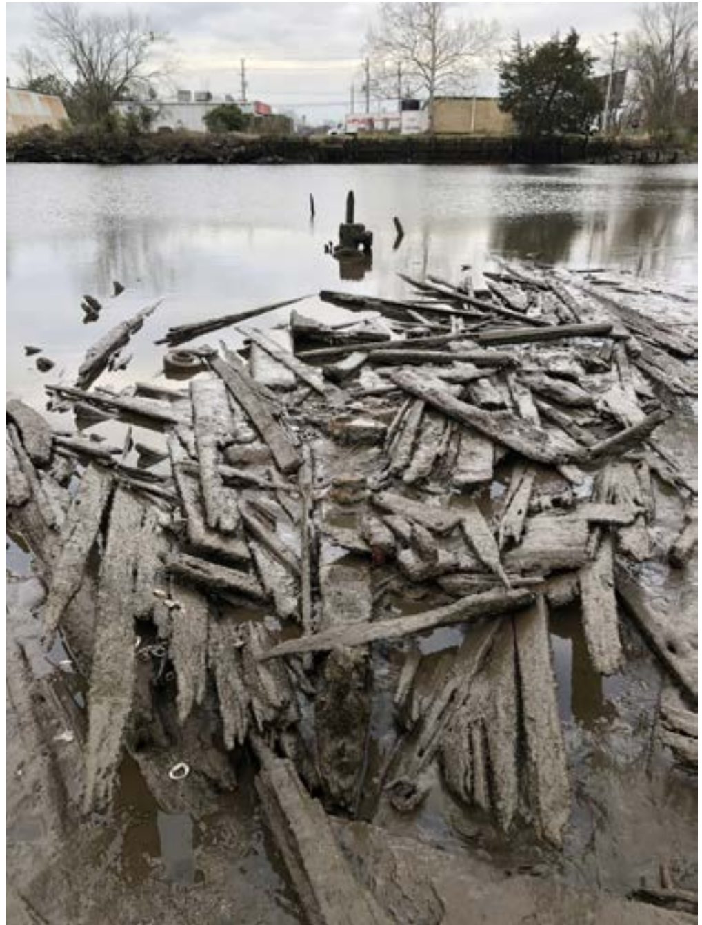
Figure 35. Vessel 6 of Feature 5, the Funkhouser Fleet. View is from bow to stern and generally to the east. Note the stem in the foreground, keelson, outer planking, and engine in the background.
