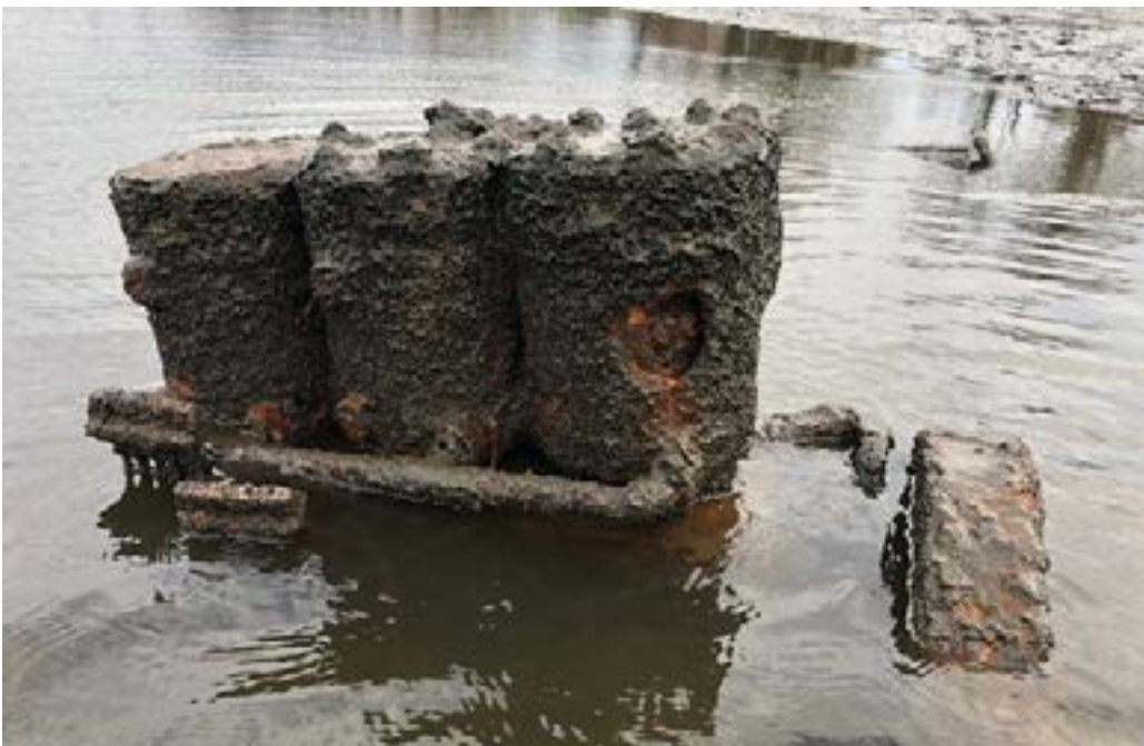
Figure 37. Three-cylinder engine on Vessel 6 of Feature 5. Note the flywheel, facing forward on the vessel.
