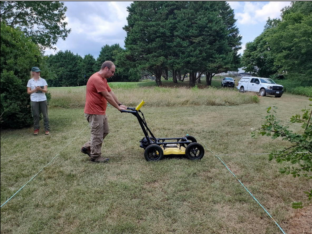
Figure #14: GPR Survey north of the Pen Park cemetery.
