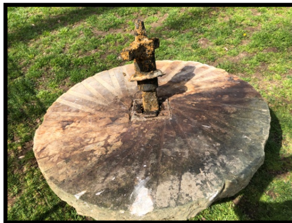
Figure 40: Second millstone salvaged from the Maury River. Note the fine dressed pattern (April 11, 2019).
